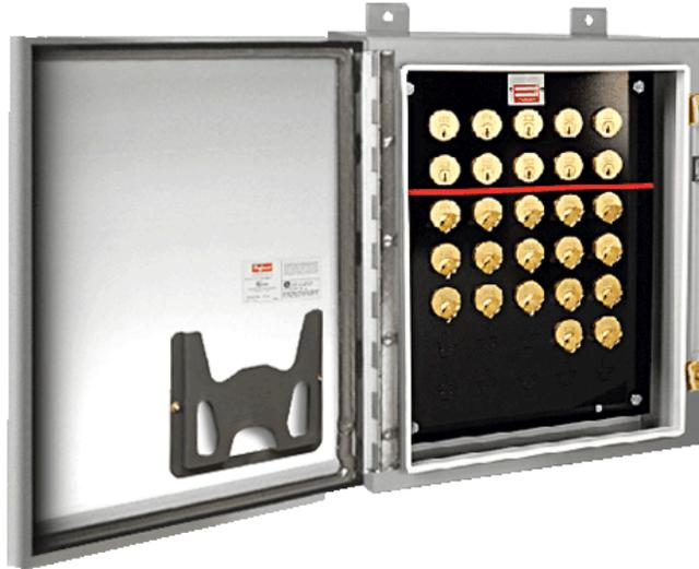
The Transfer Panel is an exchange point in which the final keys of one or more interlock sequences are exchanged for one or more different keys for additional operations. All primary (initiating) keys must be inserted into the transfer panel before any secondary (retained) keys can be turned and removed. Once a secondary key is removed, all primary keys are held captive in the transfer panel.
